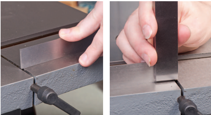
Checking both sides of the table are level
