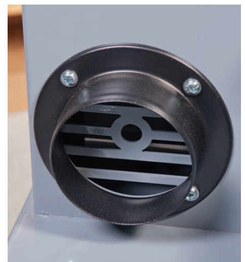
Dust extraction outlet
