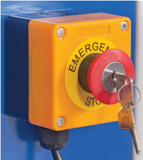
Key release emergency stop, press the button to stop the bandsaw and turn the key to release it
