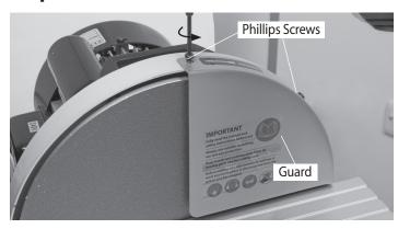
• Remove the two phillips screws that holds the guard and place them and the guard safely aside.
